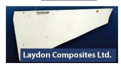
•The fastest trailer fairing install on the market! •Material is made of CRANE Composites Thermoset. •It is resilient to freezing and hot temperatures. (-60 to +190°F) •Meets EPA/CARB advanced trailer aerodynamics @ 6.67% improvement.
